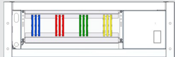
4000A/5000A system (maximum rated current of horizontal busbar: up to 5000A)
